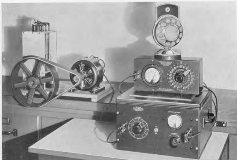
A simple assembly for noise measurement, consisting entirely of standard instruments
